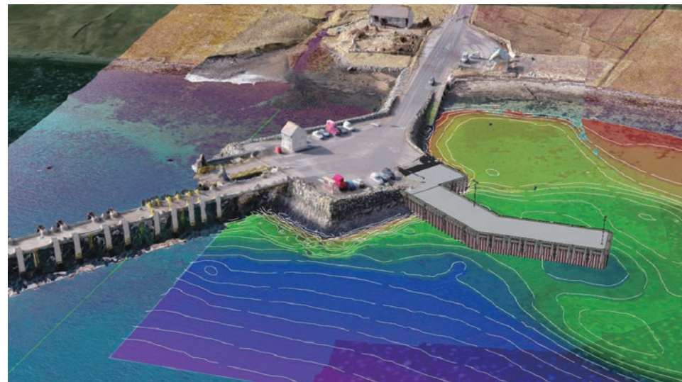
GeoBIM coordination model for the Toft Pier Development Project on Shetland
