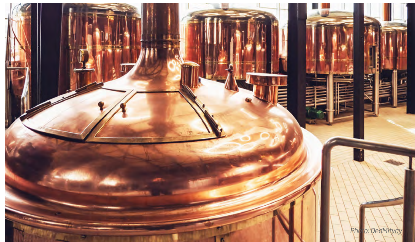
Copper tanks for beer fermentation and maturation.
