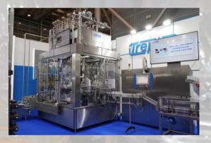
Another game-changing solution presented by Trepko was the mono-block bag in box filling system, which allow for filling and sealing in a protected atmosphere. With Trepko's Bulk Filling program already completed, this new machine moves the industries traditional bag in box system into a new era, where food saftey and hygiene is the priority.
