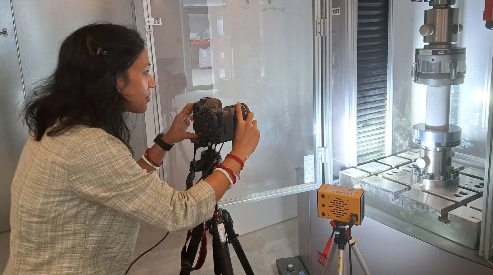
Sushree Sunayana collecting digital images during the unloading of a concrete specimen to follow the propagation of the crack pattern on the surface
