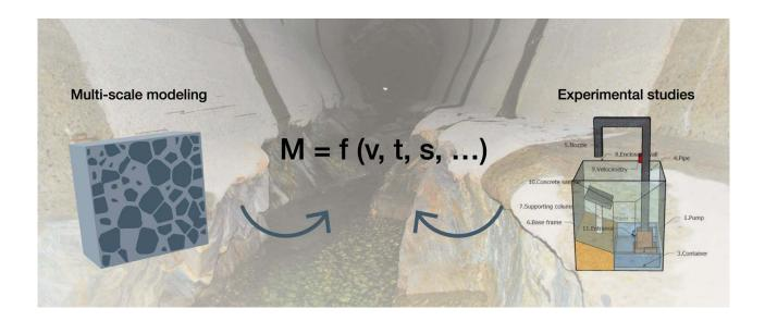
An illustration of the combined experimental and numeric studies for concrete abrasion damage in hydraulic structures
