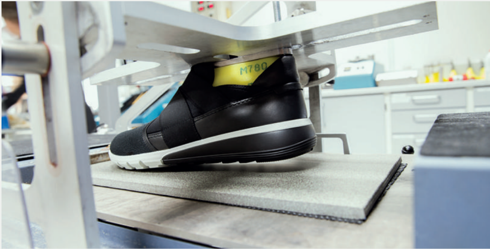
A shoe being tested for slip resistance.
