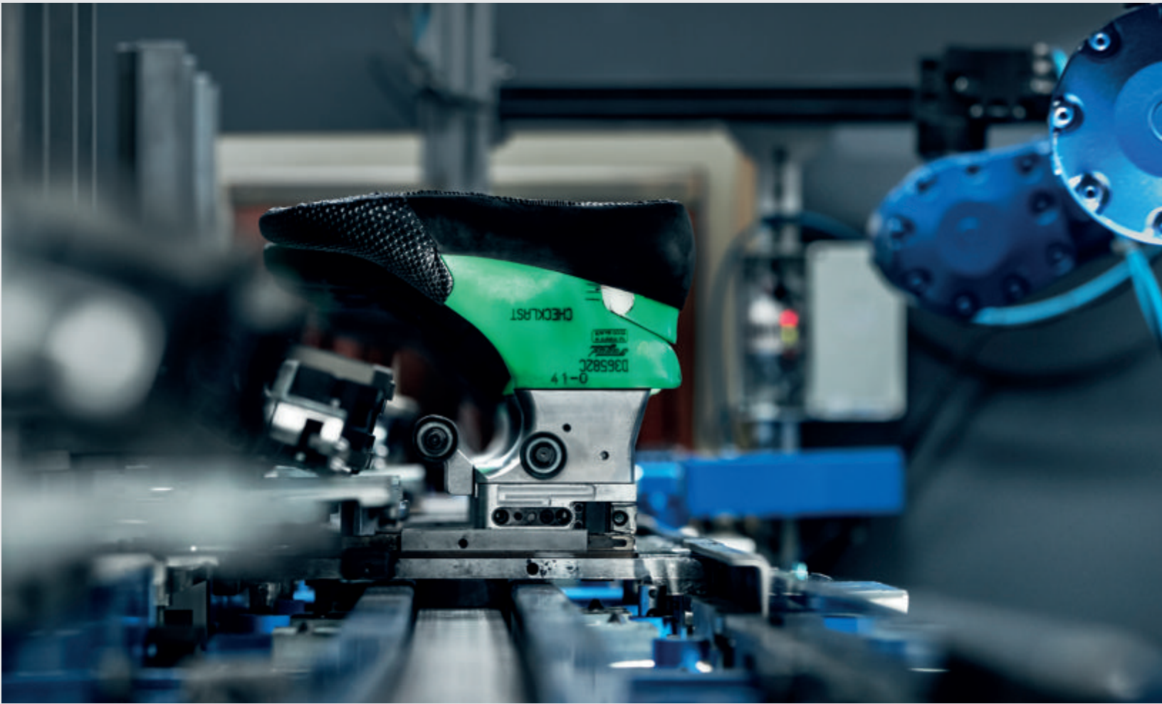
An important element of ECCO's production is the last used to shape the shoe into the perfect fit for the foot.
