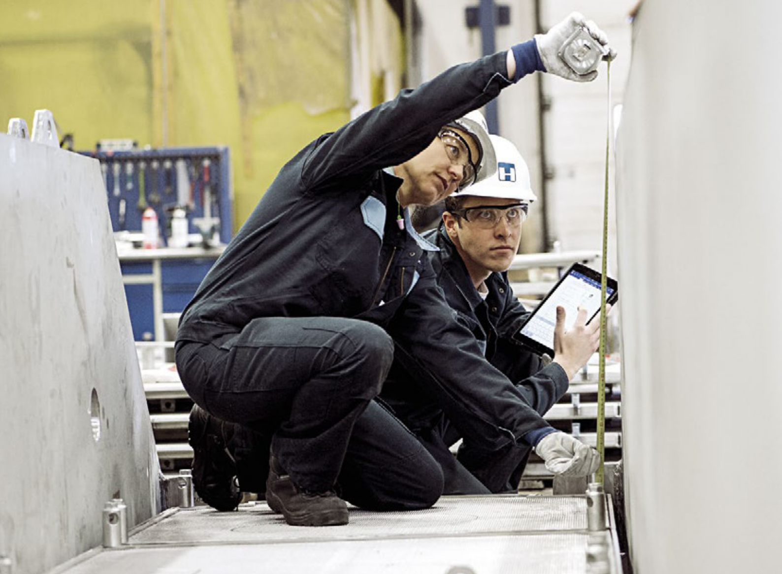
Reactor internals are inspected before shipment.
