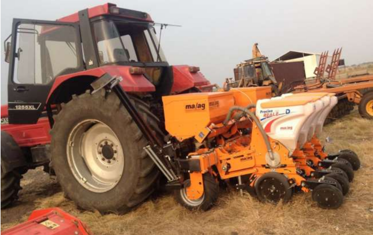
Planter from MA/AG air seeder with electronic planting control using photo cells.
