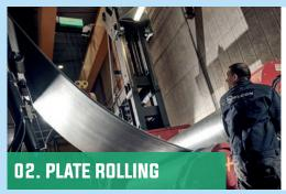
Try to roll a small sheet of metal into a perfect circle. It isn't that easy to get it just right. Now, imagine rolling a massive sheet of steel into a perfect circle of up to nine meters in diameter, where millimeter precision is essential. Quite a task, right.
