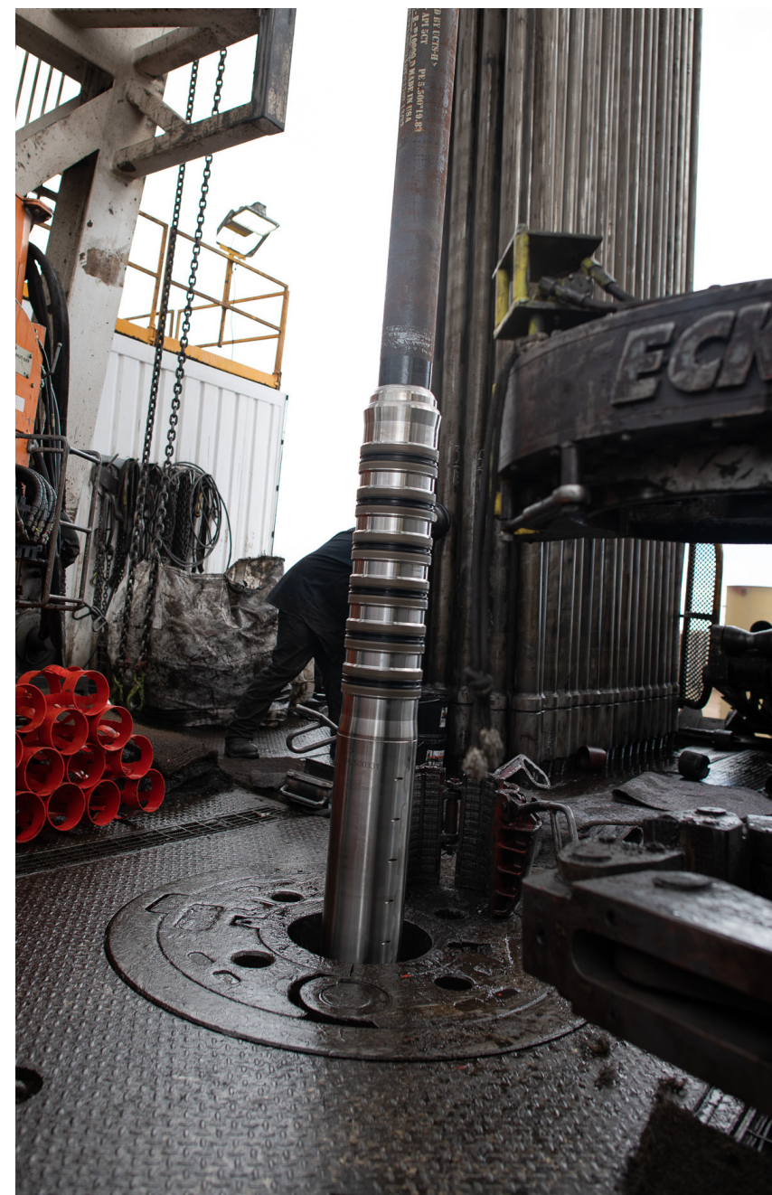
Welltec® Light Packer (WLP) being deployed for PDC Energy in Colorado, USA.
