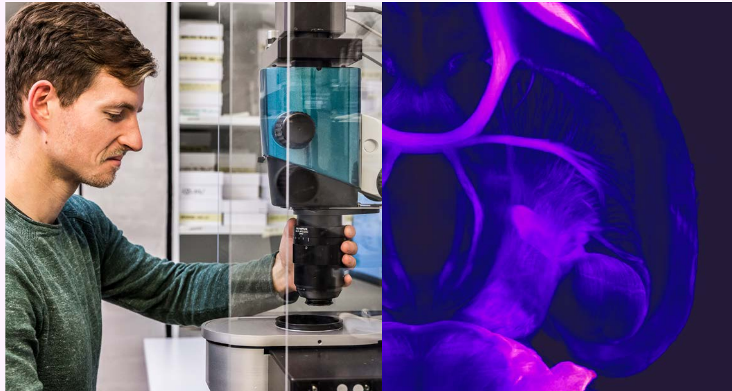
Light-sheet microscope for 3D scanning of large tissue specimens.
